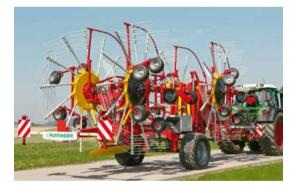
Working width is hydraulically adjustable from 26.3 to 41.0 ft / 8.0 – 12.50 m. The hydraulic drive of the front rotors enables the extending arms to be pivoted inwards for a transport height of only 13.12 ft / 4.0 m without removing tine arms or folding safety guards. Annoying setup times are therefore a thing of the past.
