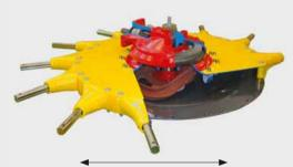
Cam track diameter 16.5 in / 420 mm
