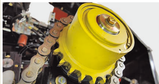
Integral Rotor protection clutch
