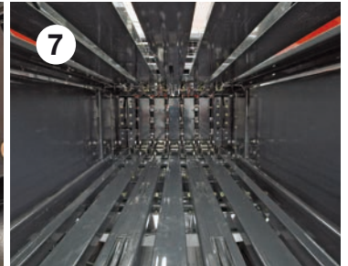
3 m (9' 10") bale chamber, with last bale ejection
