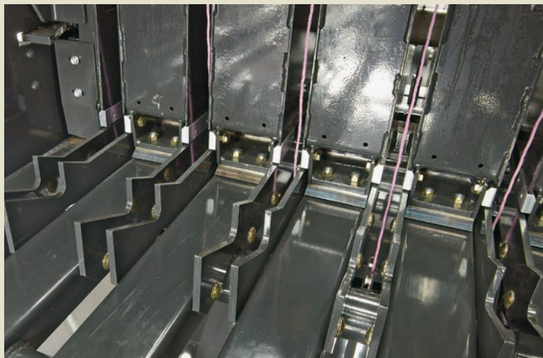
Bottom retainers prevent decompression of the bale and provide extra density
