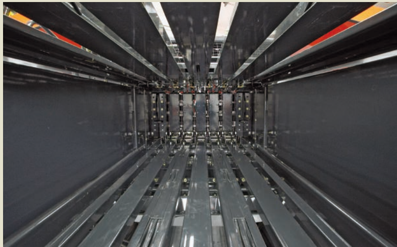
3 m (9' 10") bale chamber, with last bale ejection
