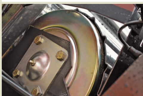
1. DIFFERENT SIZED TYRES - 2. SEVERAL HITCH OPTIONS AND A REVERSIBLE DRAWBAR - 3. BALE RAMP - 4. GREASIBLE ROLLER BEARINGS - 5. CHAIN OILER.
